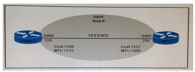
Router edge-1 is unable to establish OSPF neighbor adjacency with router ISP-1. Which two configuration changes can you make on edge-1 to allow the two routers to establish adjacency? (Choose two.)
