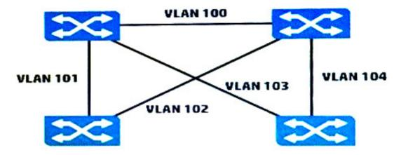
The switches in the exhibit are all HP ProVision switches that run Multiple Spanning Tree Protocol (MSTP).
